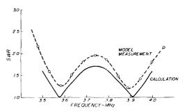
fig. 7. Calculated and measured SWR of the parallel antenna.
